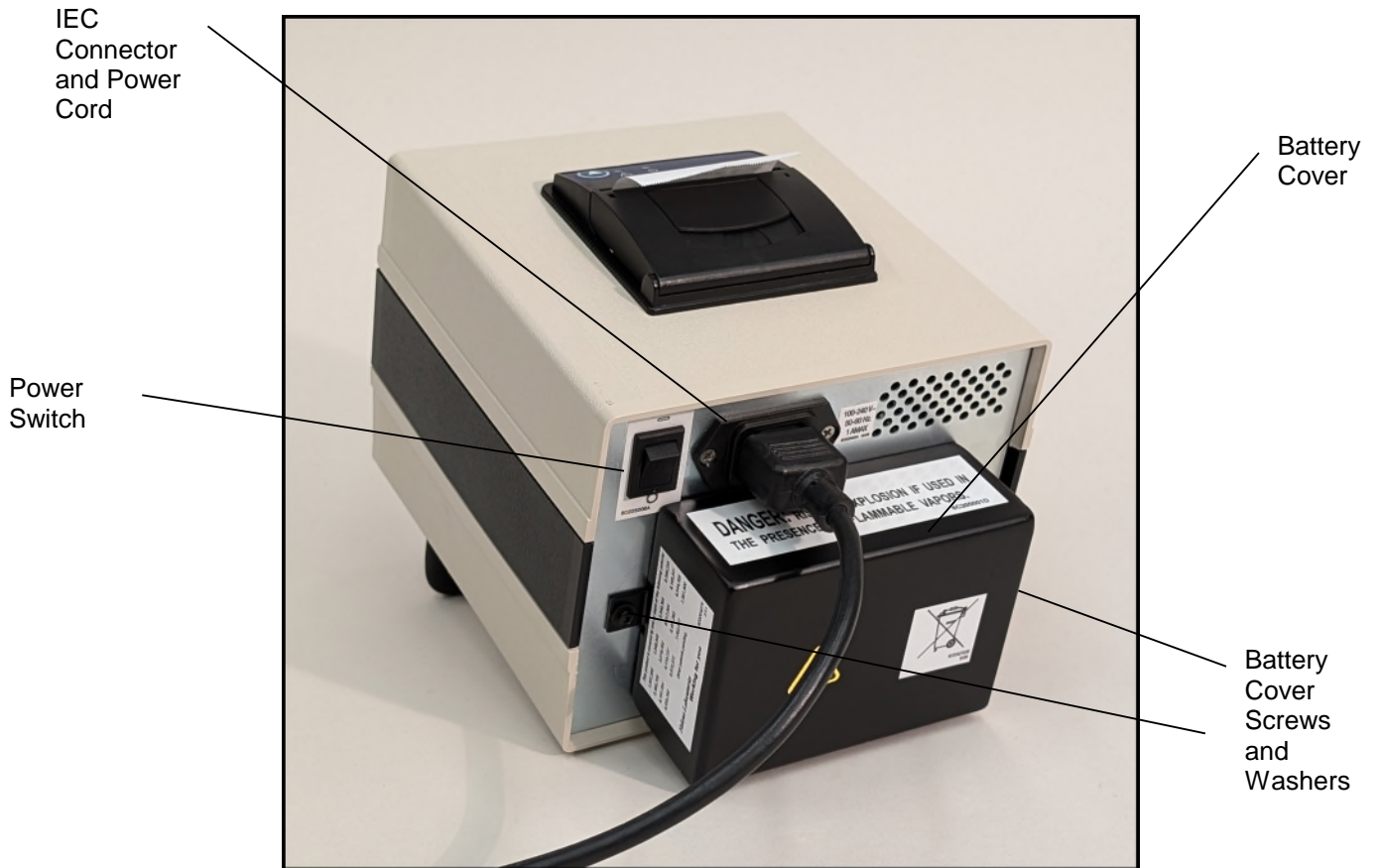
Figure 6-2. ACTALYKE MINI II with Printer, back view Back Panel Controls and Battery Access Indicated
