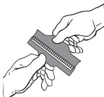
**NOTE: The Applicator Blade will only fit into the slots in the Applicator Assembly one way; do not try to force the Applicator Blade into the slots.**
