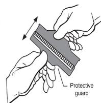
**NOTE: The Applicator Blade will only fit into the slots in the Applicator Assembly one way; do not try to force the Applicator Blade into the slots.**
