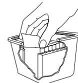
the plate in the aligning base, cellulose acetate side up, aligning the bottom edge of the plate with the black scribe line marked "CENTER APPLICATION". The identification mark should be aligned with sample No. 1.
