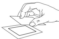
4. Apply the sample to the plate by gently depressing the applicator tips into the sample well 3 or 4 times and promptly transferring the applicator to the aligning base. Press the button down and hold it 5 seconds.
