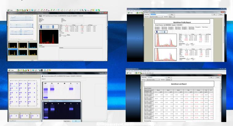
**Positive ID** – Barcoded gels allow positive ID from patient tube to final results. Using the Electrophoresis Sample Handler, QuickScan Touch can download worklists created from barcoded samples. Patient data can also be imported from LIS.
