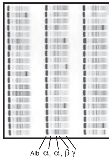
Figure 1: A SPIFE Split Beta SPE-60 Gel showing relative position of the bands.
