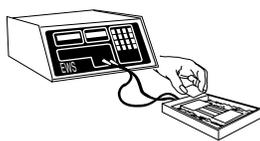
2. Place the cover on the chamber, and electrophorese the plate for 25 minutes at 350 volts.
