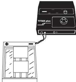
2. Electrophorese the plate(s) for 15 minutes at 180 volts. Power must be applied within 5 minutes after the plate(s) has been placed in the chamber.
