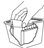
the plate in the aligning base, cellulose acetate side up, aligning the bottom edge of the plate with the black scribe line marked "CENTER APPLICATION". The identification mark should be aligned with sample No. 1.
