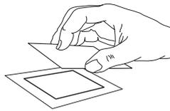
4. Apply the sample to the plate by gently depressing the applicator tips into the sample well 3 or 4 times and promptly transferring the applicator to the aligning base. Press the button down and hold it 5 seconds.
