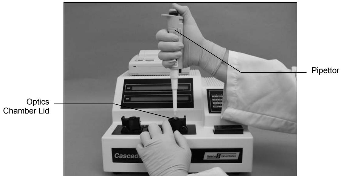
**Fig. 6-2. Simultaneously Press Optics Chamber Lid and Pipette Reagent**
