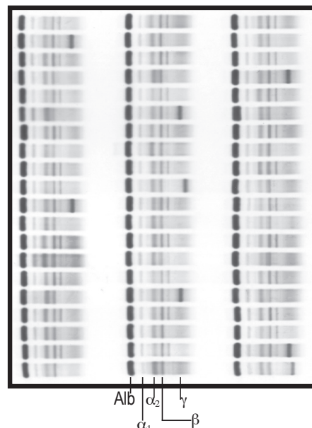
Figure 1: A SPIFE Split Beta SPE-60 Gel showing relative position of the bands.
